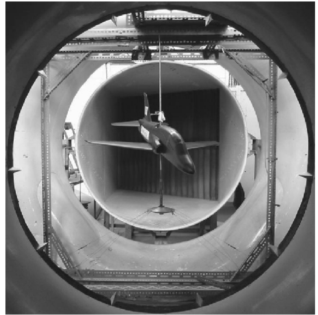
Fig. 2 Dynamic wind-tunnel rig with a one-twelfth scale BAe Hawk model.
